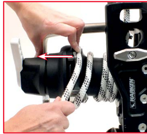
10. Fit the rope into the rope grab. Raise the cover to make this easier.
