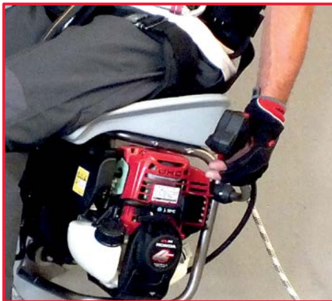
8. Adjust the position of the accelerator control so it is ergonomically comfortable for the operator and away from the engine exhaust. To do this, loosen the fixing screw, position the accelerator control and retighten the fixing screw.
