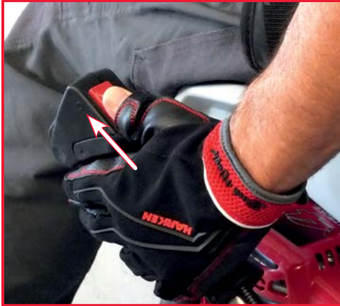
1. Switch off the engine by moving the accelerator control to the " 0 " position.
