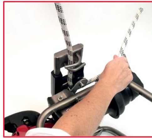
6. Pass the rope round the pulley.
