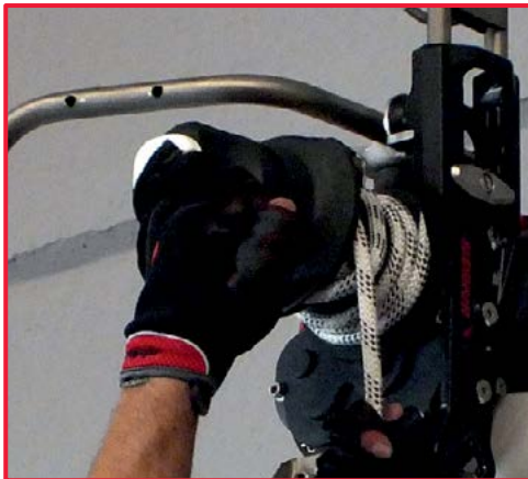
3. With the other hand, turn the control lever clockwise to allow the rope to slip on the winch drum and permit a controlled descent. To adjust descent speed, manually control the speed at which the rope leaves the winch. To stop the descent, release the control lever.
