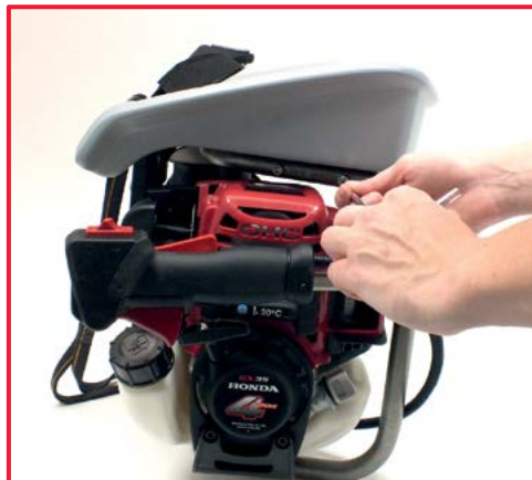
2. Unscrew the four screws that fix the seat to the chassis with a n°5 hex Key.
