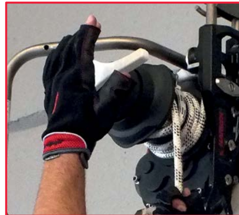
3. With the other hand, turn the control lever clockwise to allow the rope to slip on the winch drum and permit a controlled descent. To adjust descent speed, manually control the speed at which the rope leaves the winch. To stop the descent, release the control lever.
